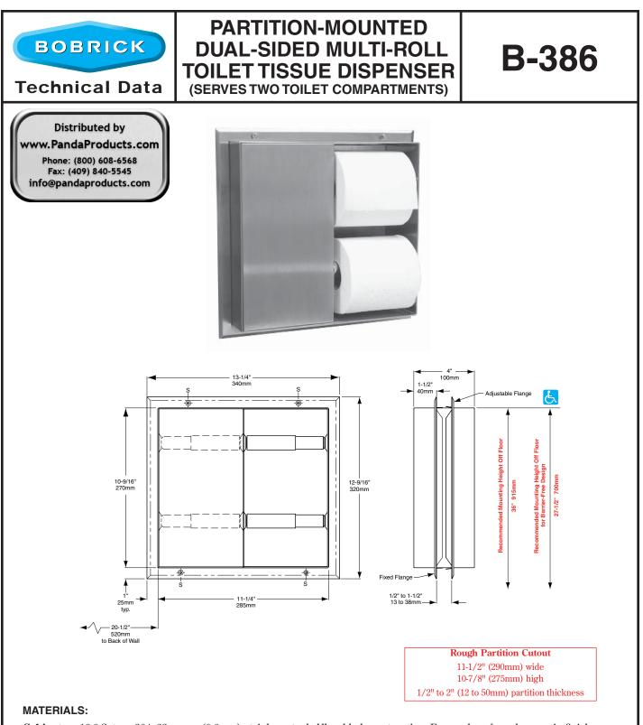
**Cabinet** — 18-8 S, type-304, 22-gauge (0.8mm) stainless steel. All-welded construction. Exposed surfaces have satin finish. **Flanges (2)** — 18-8 S, type-304, 22-gauge (0.8mm) stainless steel with satin finish. Drawn and beveled, one-piece, seamless construction.
