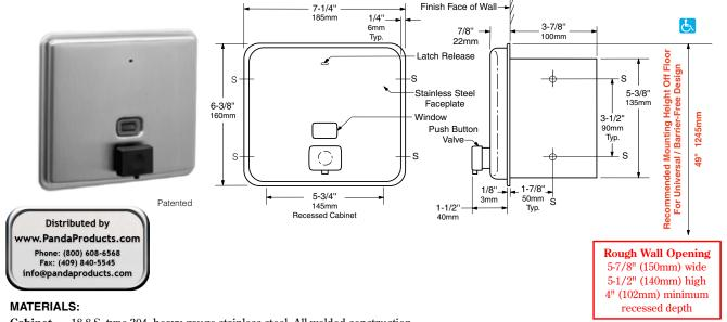
Cabinet — 18-8 S, type-304, heavy-gauge stainless steel. All-welded construction.
